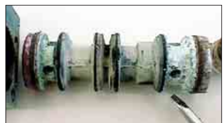
Contaminants corrode and damage air-operated equipment
